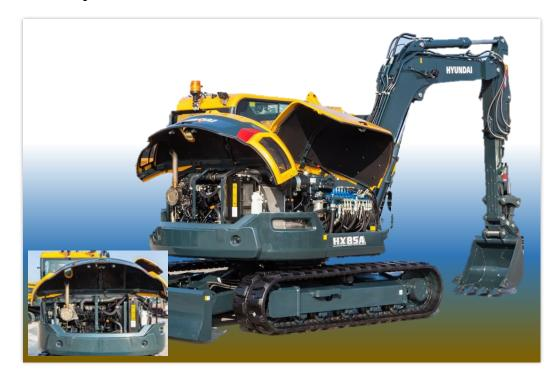
The HX85A has a large rear engine hood and side cover, that opens wide to allow for easy daily maintenance and give excellent access to service areas. Wear parts that require regular replacement, such as filters are conveniently positioned and easy to reach from the ground.
