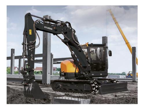
A brand new 2-piece boom gives the midi excavator an all-dynamic working range and considerable flexibility. It allows the machine to extend the maximum reach of the arm as well as working very close to its own tracks. Effective vertical digging becomes natural, same as an impressive overloading height.
