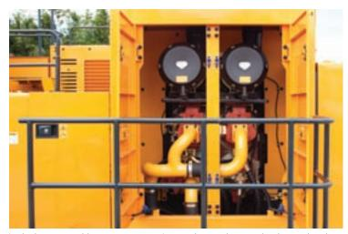
To achieve optimum precision, Hyundai redesigned the hydraulic system to provide the operator with super fine touch and top level controllability. Spool valves in the control valve are engineered to provide more precise flow to each function with less effort. Improved hydraulic valves, variable volume piston pumps, fine-touch pilot controls and enhanced travel functions make any operator look like a smooth operator. Newly improved features
